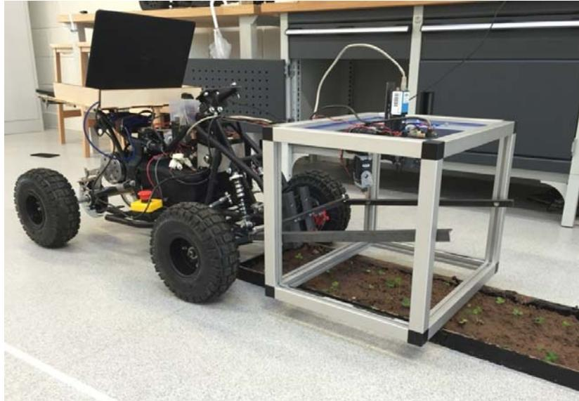
**Fig. 1.** The laser weeding robot.
