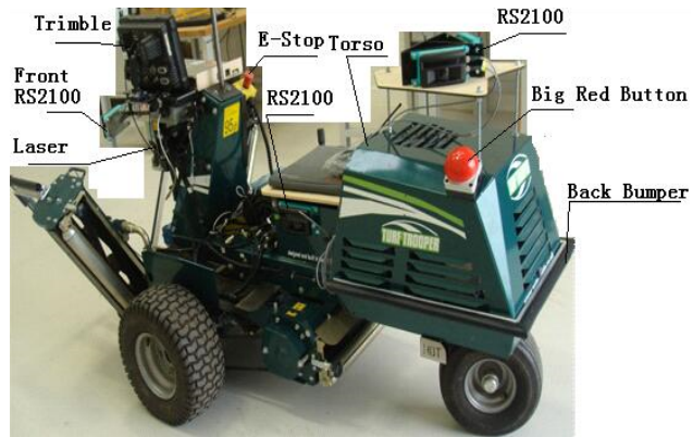
Figure4.1. Design and Build Six RS2100 Distance sensors for safety system about TOMI Robot
