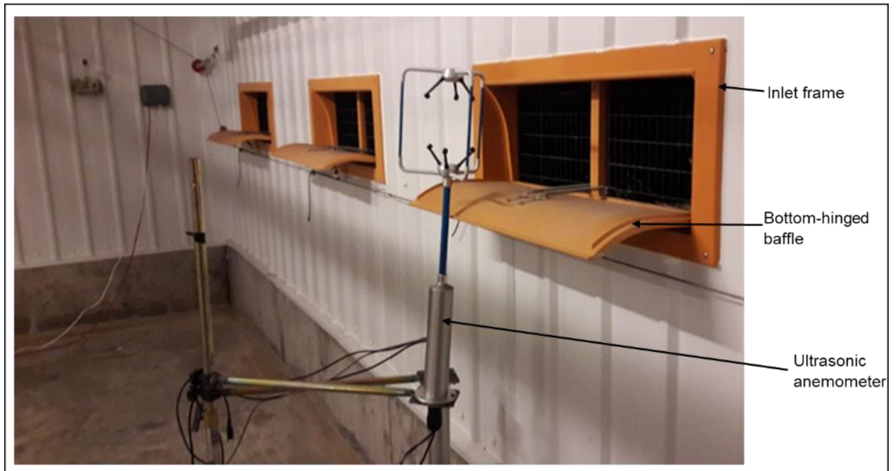
Figure 3.3: Airspeed measurement at the air inlet of an experimental broiler building
