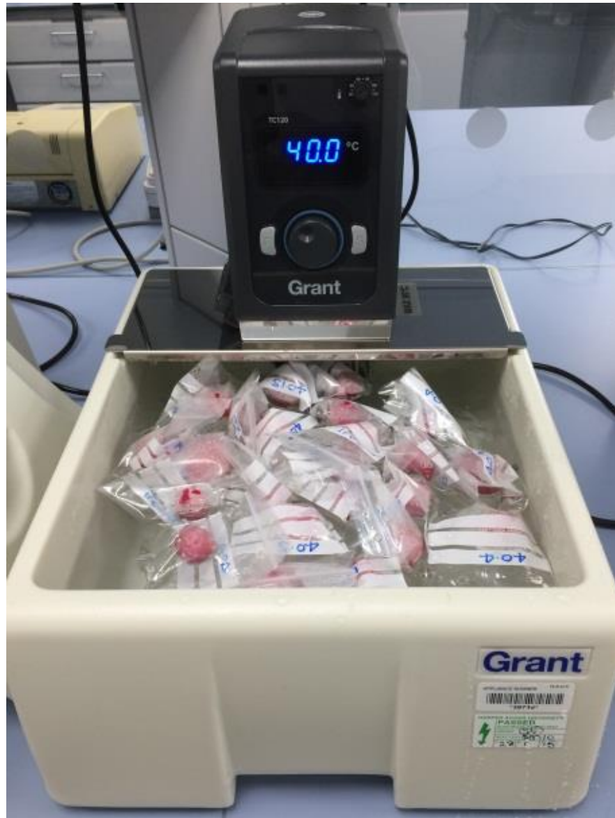
Figure 4-25 Water bath set to 40°C containing radishes in grip seal bags prior to texture analysis
