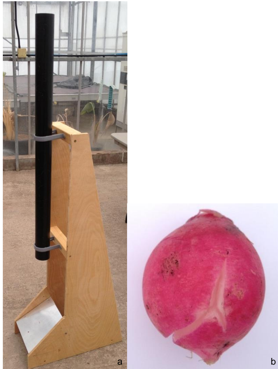
Figure 2-14 Impact texture analysis of a radish hypocotyl from a height of 1.4 m onto a metal plate (a) resulting in a split radish (b)
