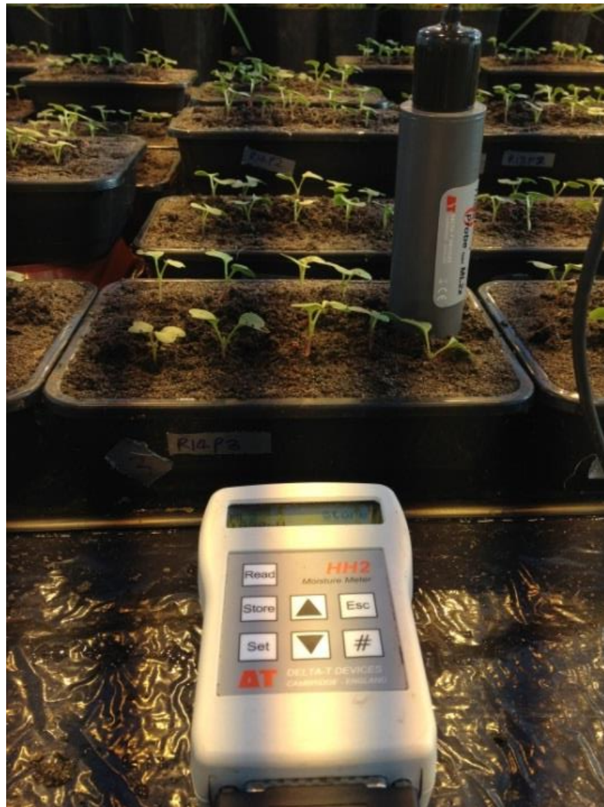
Figure 2-4 The VWC of the compost in a plant pot was measured using a Theta Probe (Delta T Devices, Cambridge, UK). In this picture the prongs of the Theta Probe are fully inserted in the compost.
