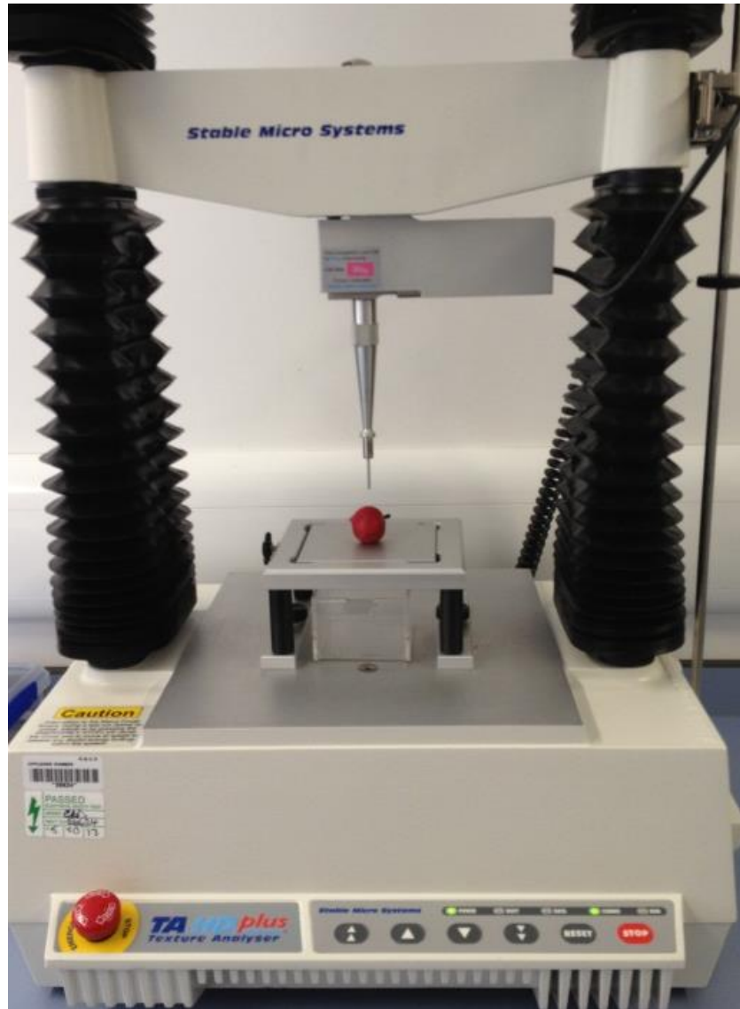
Figure 2-11 Texture analysis of a radish using TA.HD.plus texture analyser (Stable Micro Systems, Surrey, England).
