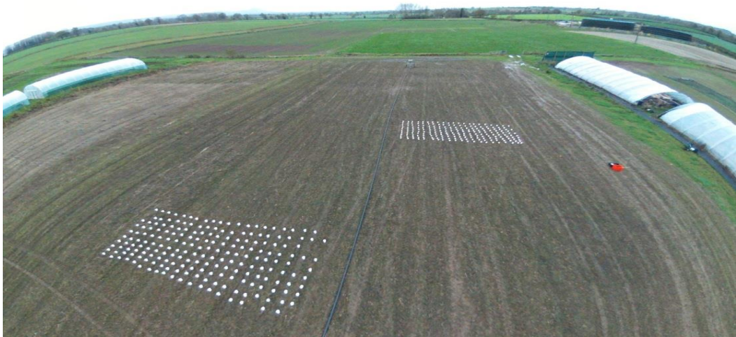
Figure 4. 5 Aerial view of the placement of the catch cans for the boom irrigation system in the field (Source: obtained from Grove, 2015)
