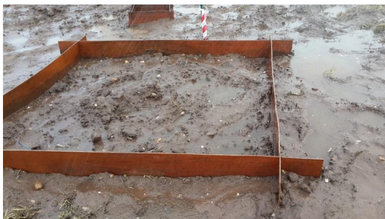
Figure 6. 13 Sprinkler irrigation process over water-runoff sampler
