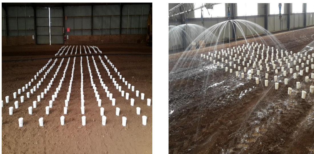
Figure 4. 4 Catch cans distribution and water distribution uniformity test in soil hall
