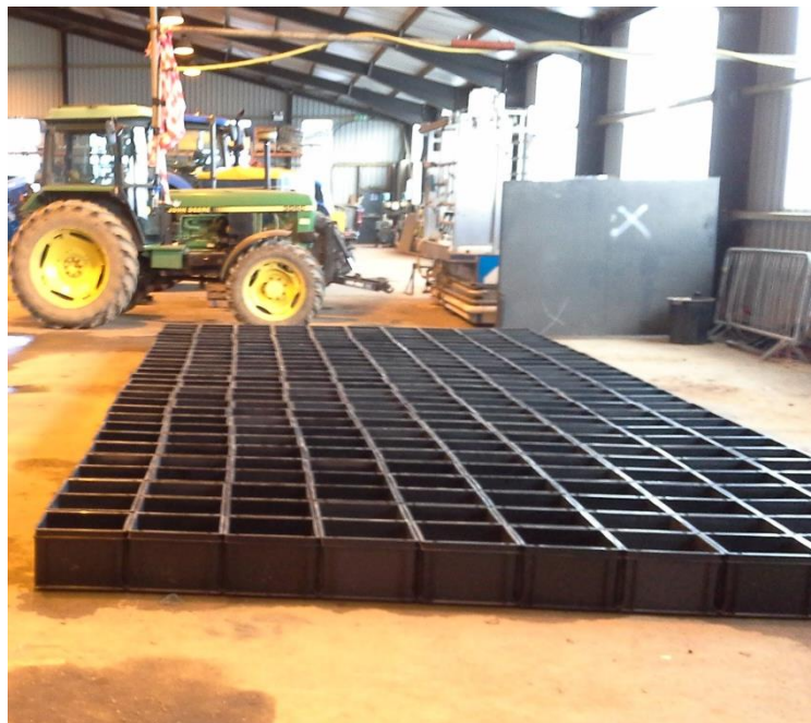
Figure 3. 5 Water distribution uniformity tests of a sprinkler using rectangular cans
