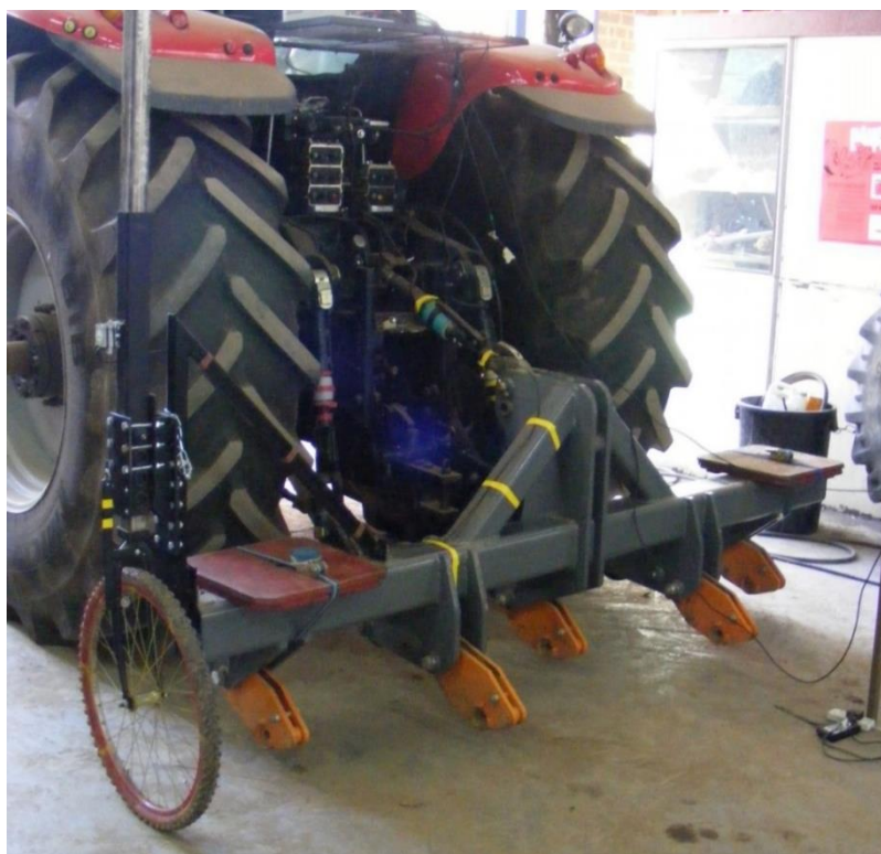
Figure 63: Linkage control evaluation experiment test set up
