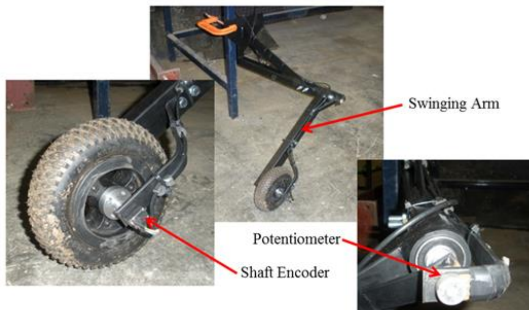
Figure 28: A swinging arm depth wheel suitable for measuring axle vertical displacement and forward speed
