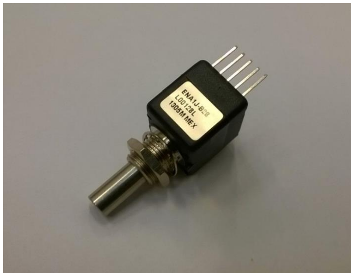
Figure 49: Bourns EMA1J-B20 optical end encoder used in this study
