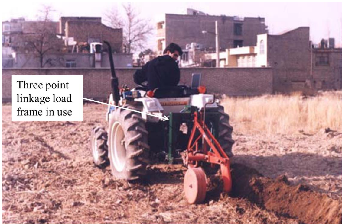
Figure 22: A typical linkage mounted load frame in use
