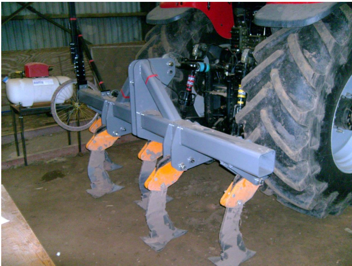
Figure 55: Wing tined 1, 2, 3, or 5 leg sub-soiler developed for this study
