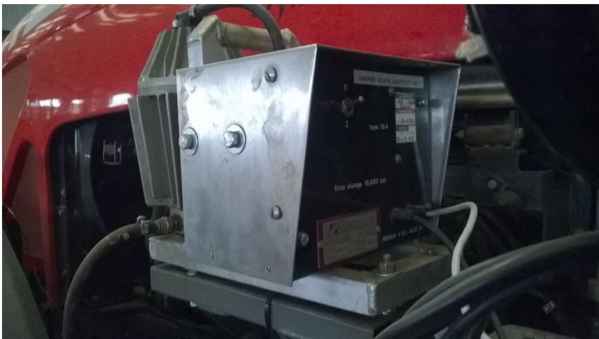
Figure 52: JPS Engineering FMS MK4 fuel measuring system fitted to the MF8480 research tractor
