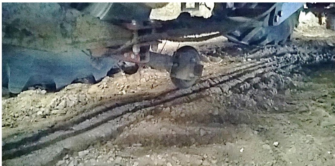
Figure 39: Image of the front axle height sensor fitted to the MF8480 research tractor
