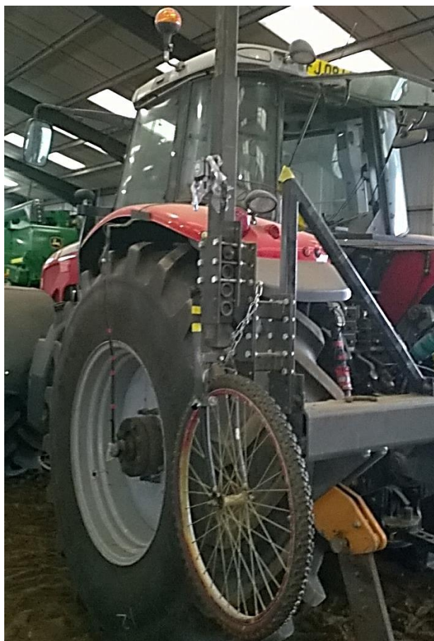
Figure 33: Measured implement tillage depth (AID) measurement wheel used
