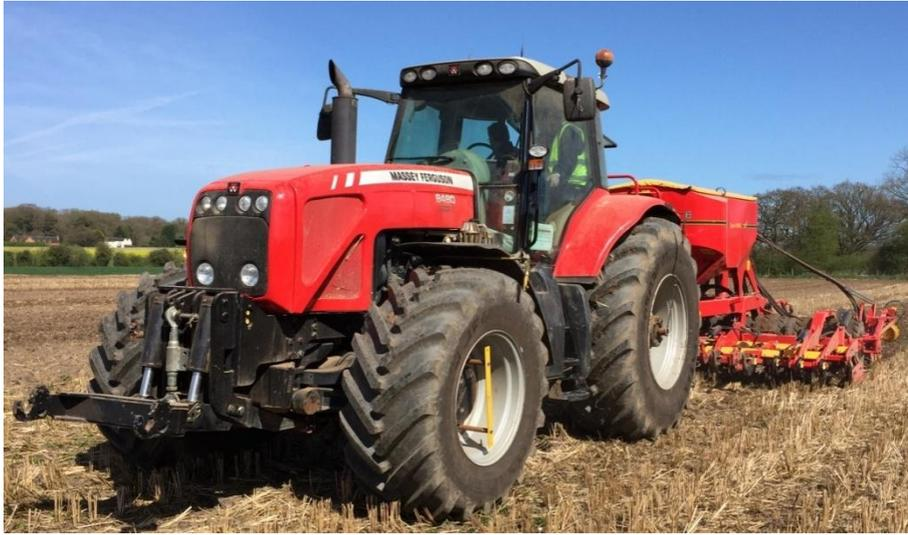
Figure 3.6 - Massey Ferguson 8480 (216.3 kW [290 HP]; 12.5 tonne) tractor
