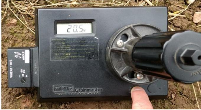
**Figure 6.12 - Protimeter Grainmaster grain moisture meter**
