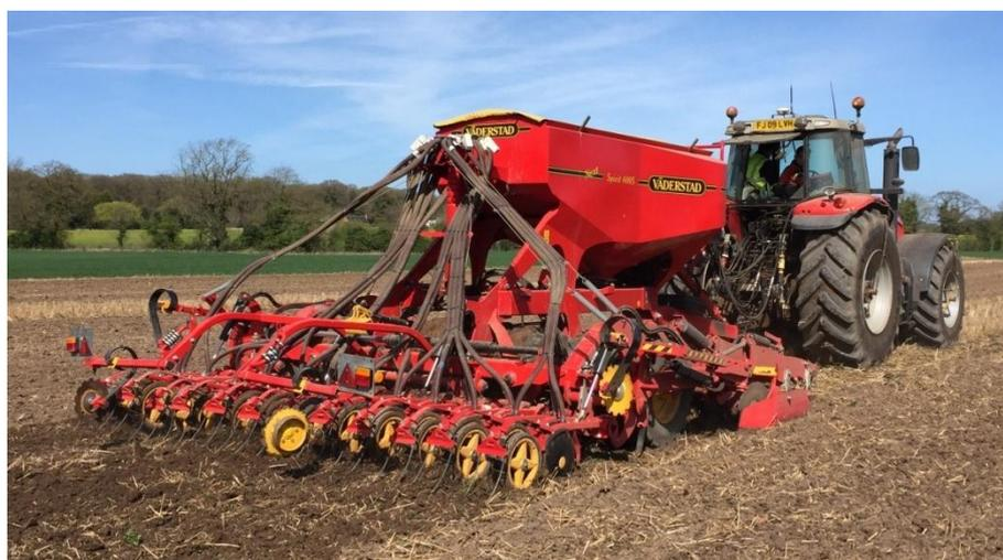
**Figure 3.11 - Väderstad 4 metre Spirit drill pulled by the Massey Ferguson 8480 tractor**
