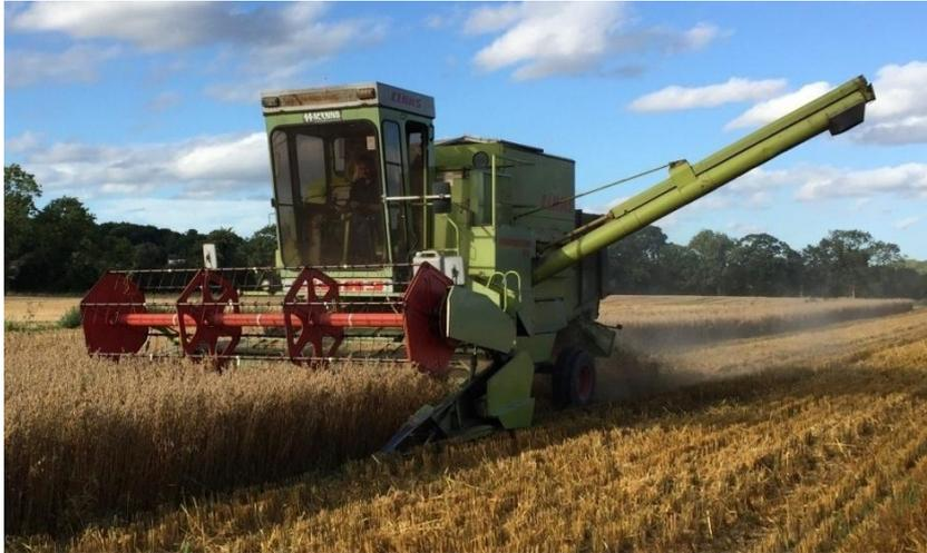
**Figure 6.9 - Claas Dominator 85 combine harvester with a 4 metre cutter bar**
