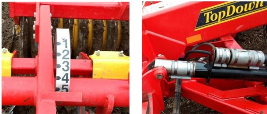
**Figure 3.10 - Implement depth settings on the Väderstad Topdown left: indicators and right: packers**
