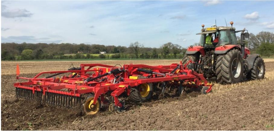
**Figure 3.9 - Väderstad 4 metre wide Topdown cultivator pulled by the Massey Ferguson 8480 tractor**
