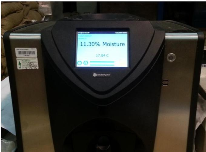
Figure 6.5 - Dickey John Grain Analysis Computer (GAC) 2500-UGMA
