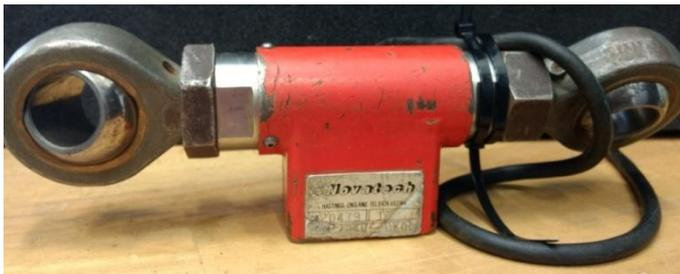
**Figure 6.11 - Novatech F204TFROKO 1 tonne strain gauge**
