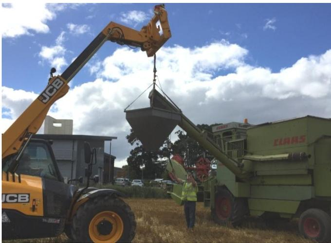
**Figure 6.10 - Weighing grain with a hopper and 1 tonne load cell**
