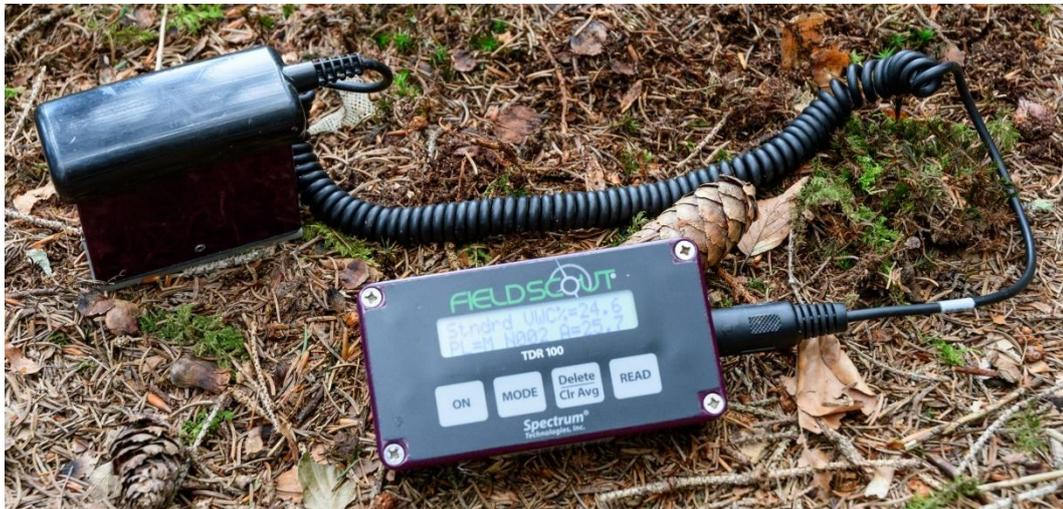
**Figure 4.6 - Spectrum Field Scout TDR 100 soil moisture meter**
