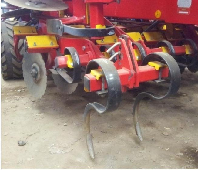
**Figure 9.2 - Wheel track eradicator tines fitted to Väderstad Spirit pneumatic seed drill**
