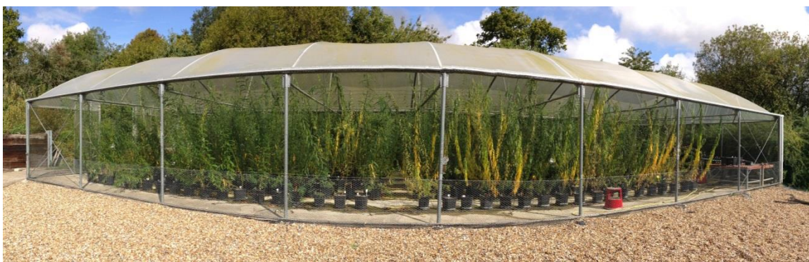
Figure 2.4 The open south facing side of GH44, the rain out shelter that housed the pot experiment.
