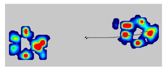
**Figure 2.** Tekscan 'heatmat' visualisation of peak vertical landing force (N). Colours provide a visual representation of measured forces from low (blue) to high (red). The black and white symbol indicates the centre of gravity at the point of measurement.
