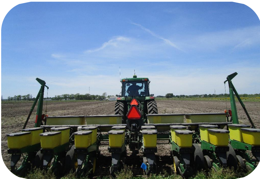
Figure 3.4c. Seed planting in mid-May (Planter model: JD 7200 Max Emerge 2)
