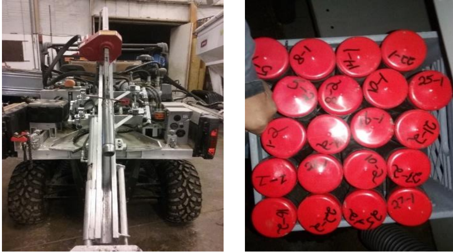
Figure 4.2. Gator mounted Giddings machine (left) and soil cores (right) collected for X-ray CT scanning.
