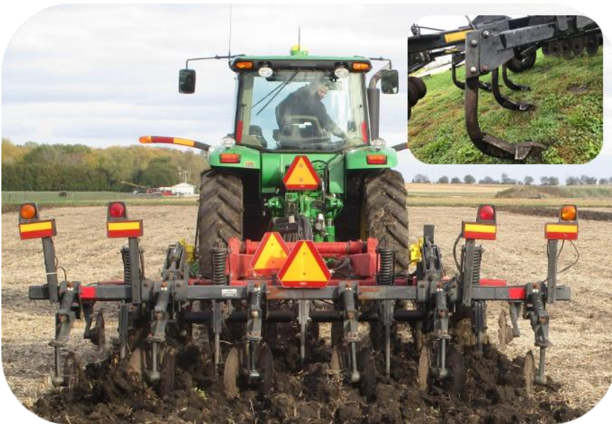
Figure 3.4a. Deep tillage operations during fall after harvest of crops (Disc ripper model: CASE/IH ET 527B). Tines used are shown top corner of the picture.
