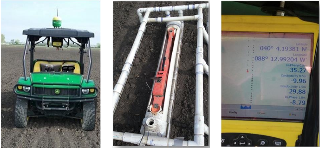
Figure 3.12. JD Gator, Veris EM38 Sensor and data recording for EC measurement
