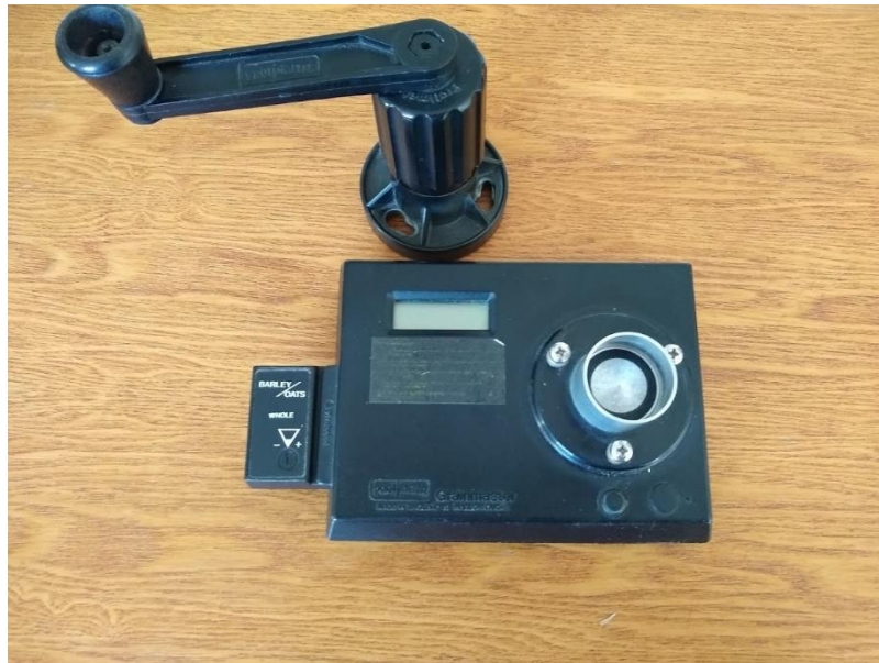
Figure 6.4 Grainmaster protimeter for assessing grain moisture during harvest
