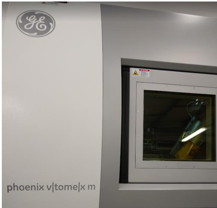
Figure 4.4 Phoenix v|tome|x m X-ray microfocus CT system
