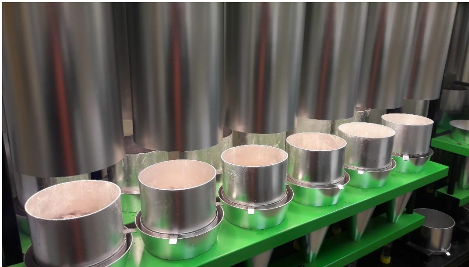
Figure 5.2 Tullgren funnels used for extracting springtails
