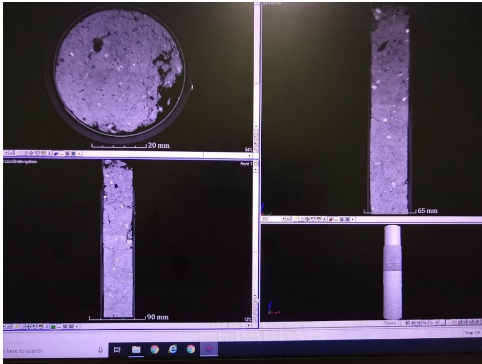
Figure 4.5 Top view (upper left) and side view (bottom left and top right) of combined X-ray CT scans in VG Studio
