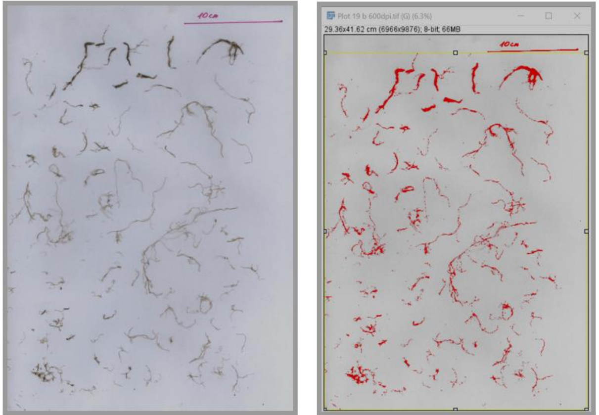
Figure 6.2 View of roots scan on the left and the same picture after applying Otsu thresholding in Image J Fiji processing on the right.
