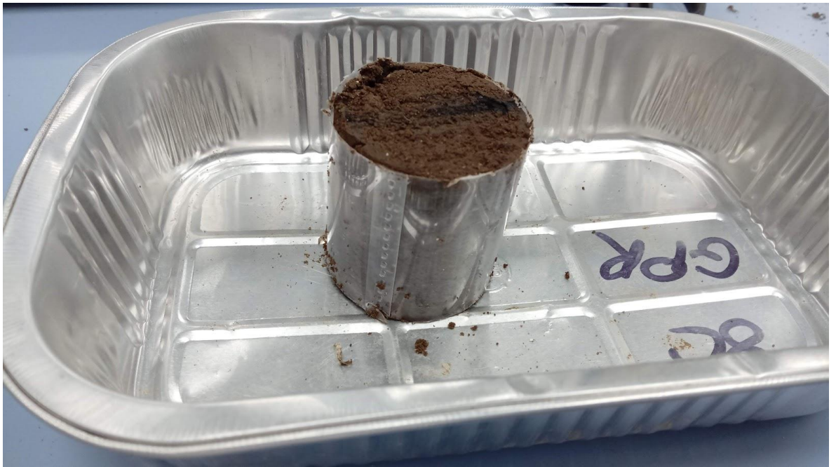
Figure 4.2 50-mm long slice of soil after cutting to measure soil bulk density
