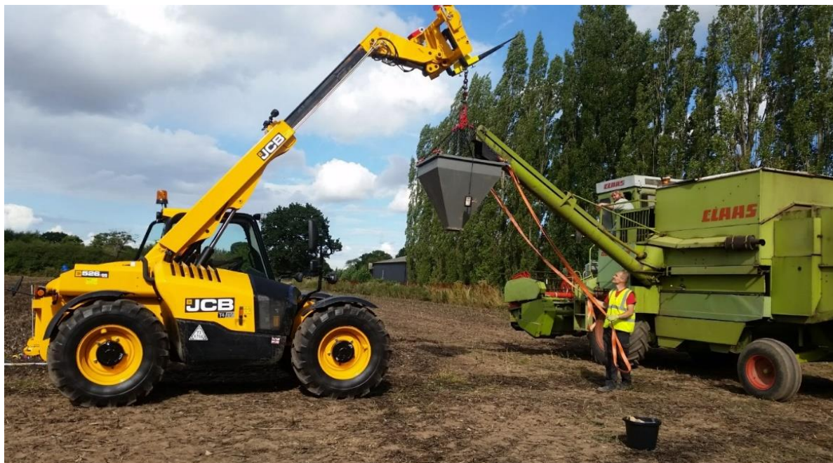
Figure 6.3 JCB telehandler with an external hopper and a loadcell for weighing the yields
