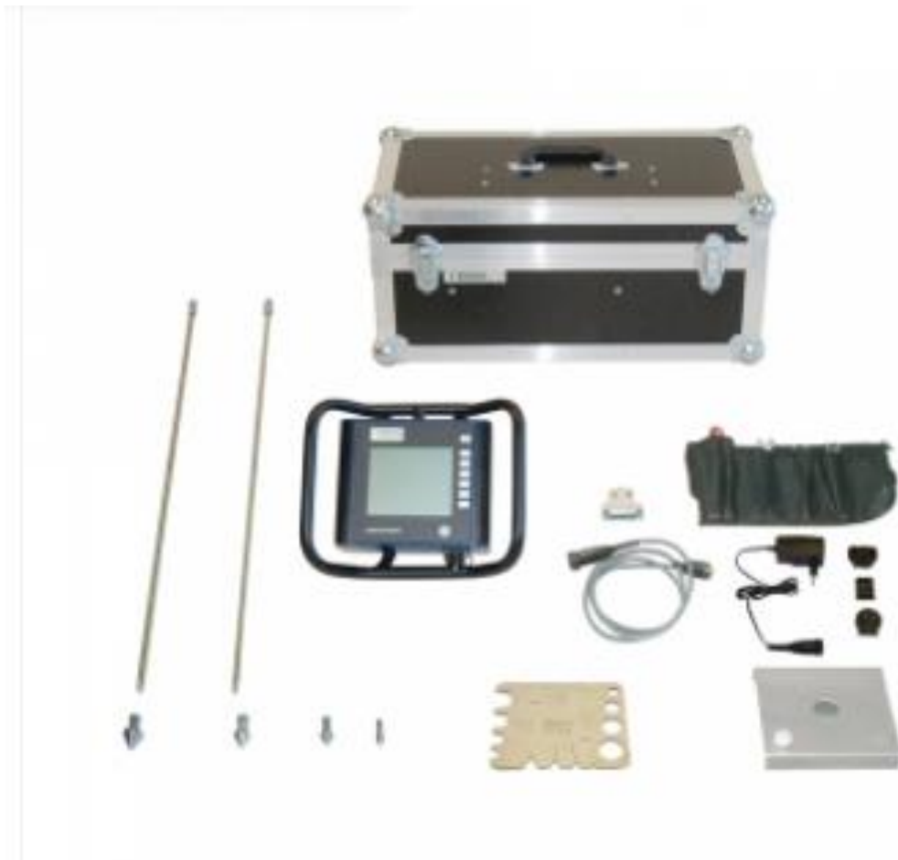
Figure 4.3 Eijkelkamp 06.15.31 Penetrologger set (Source adapted from Eijkelkamp, 2021).
