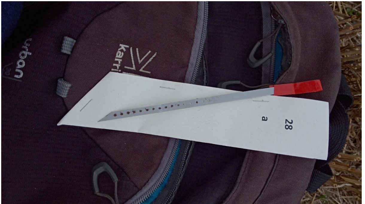
Figure 5.1 Bait lamina stick after collection from the soil
