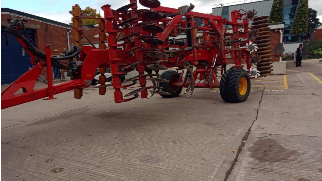
Figure 3.8 The Top Down 400 implement used for tillage on the Large Marsh experiment.
