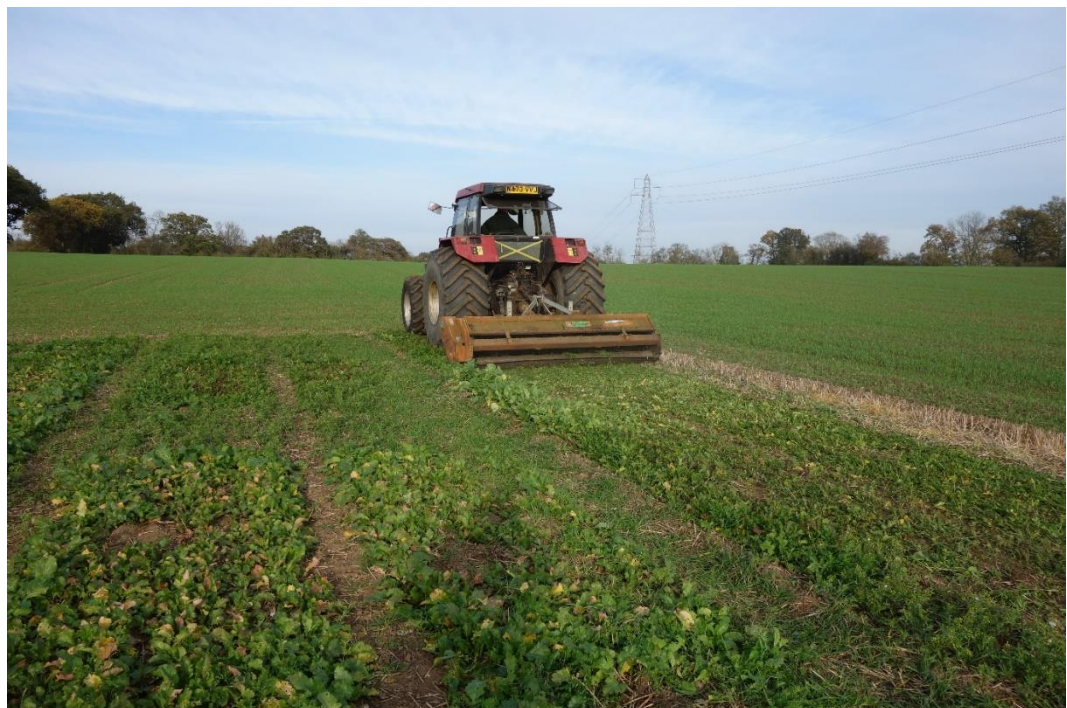
Figure 6.4. Case IH 5150 tractor operating a flail mower (RMU 290, Agrimaster) to macerate brassica plants in field experiment 1 (Malvern, Worcestershire, UK)
