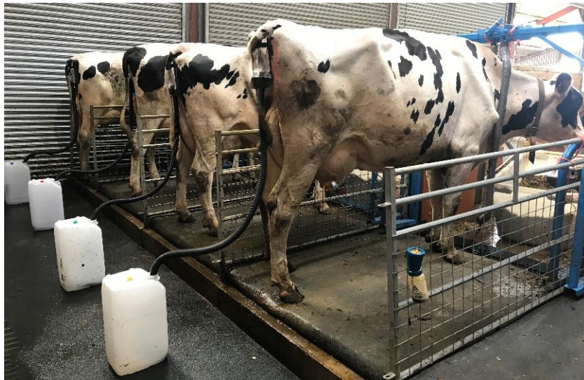
Figure 3.1: Urine collection apparatus including storage barrels
