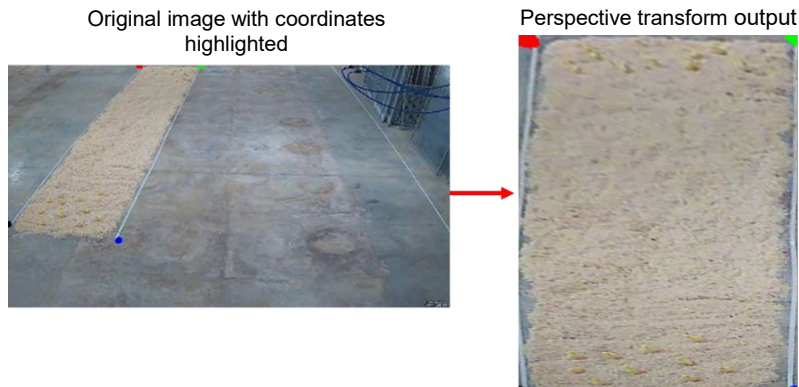
Figure 8. An example of Perspective Transform conducted in the angled camera experiment.
