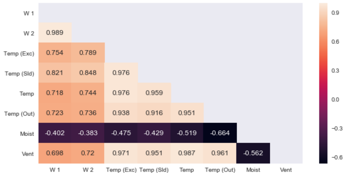
Figure 5.1: The correlation matrix for all sensors. W1 stands for water sensor at Drinker 1, while W2 stands for water sensor at Drinker 2. Temp stands for temperature, moist stands for moisture, and vent stands for ventilation. Exc represents the temperature of the excrement area, sld represents the temperature of the solid area and out represents the outside temperature.
