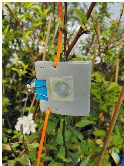
Figure 6.6- An enclosure made to isolate Woolly Apple Aphid ( Eriosoma lanigerum ; WAA) nymphs on apple material in outdoor settings or on larger plants. This enclosure is a modification of a standard clip cage design, developed to fit around woody material. It is constructed of two sheets of 10 mm thick EVA foam (80 mm × 80 mm) joined with contact cement on the right-hand side. A 25 mm × 25 mm window was cut in one piece and covered with fine mesh, ca. 50 - 100 μm and secured with contact cement, to allow viewing of the aphid colony and air flow, but to prevent nymphs from escaping. The cage can be placed around a WAA colony feeding on woody material and secured so that it sits tight to the stem with for instance bulldog clips and cable ties, as shown in the figure, depending on the diameter of the woody material.
