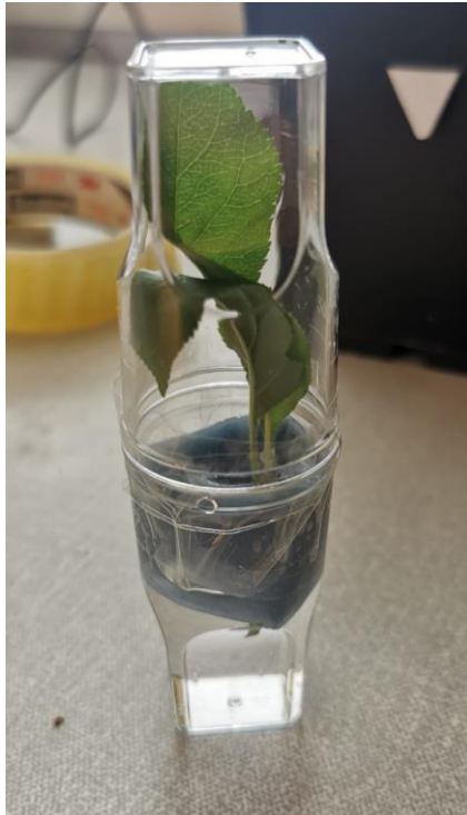
Figure 6.2 - Experimental enclosure set up to isolate individual Woolly Apple Aphid ( Eriosoma lanigerum ; WAA) nymphs for life history studies. Each enclosure consisted of two plastic pots, inverted, and secured together with electrical tape (clear sticky tape in this image). Containers were ca. 30 mm diameter in the centre, 20 x 20 mm base, 55 mm in height each (110 mm total height). A piece of floral foam the diameter of the containers was cut and soaked in water. A small reservoir of water was filled underneath the floral foam such that the end of the petiole cutting can reach the water. The floral foam functions to prevent aphids from drowning in the water and maintains humidity for the leaves. Enclosures were arranged in a complete randomised design within a growth room.
