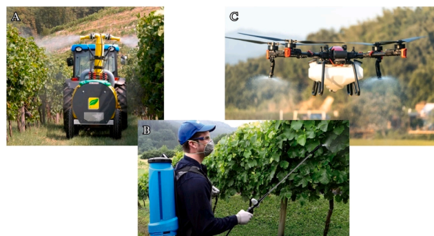
Fig. 1. Pesticide spraying equipment used across scenarios: (A) the Caffini Smart Synthesis Hybrid vine sprayer [66,71]; (B) a backpack sprayer [67,72]; and (C) the XAG P100 spray drone [68,73].
