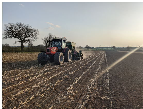
Figure 3.8: A SAME Iron 165.7 tractor (163 HP) equipped with a John Deere 750a drilling spring beans (var. Lynx) on 28/03/2022 Source: Author's own
