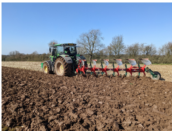
Figure 3.7: John Deere 6250R (250HP) with a six furrow Kverneland plough establishing the CON treatment on 19/03/2022. Source: Author's own
