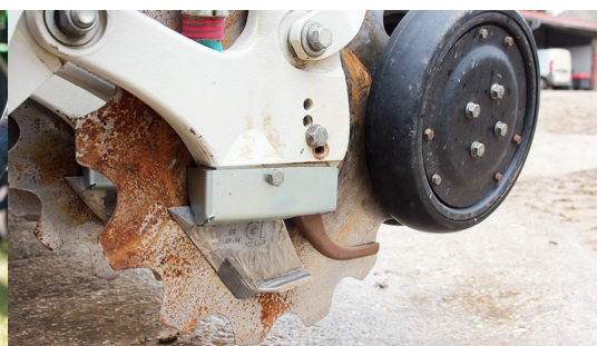
Figure 2.12: An example of a disc opener. Source: Oliver (2017)
