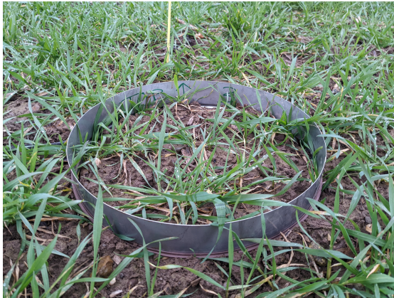
Figure 7.2: The static chamber base, which remained in the soil for the duration of the sampling period. Source: Author's own
