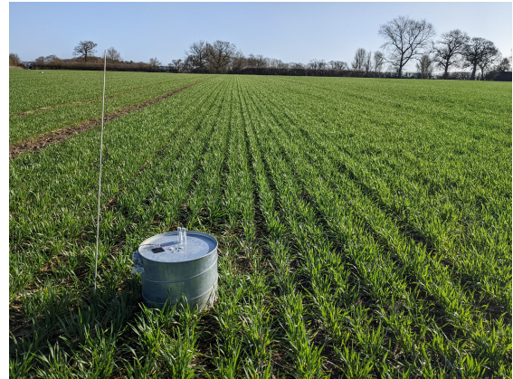
Figure 7.3: The static chamber top, which was placed onto the chamber base during individual samples. Source: Author's own
