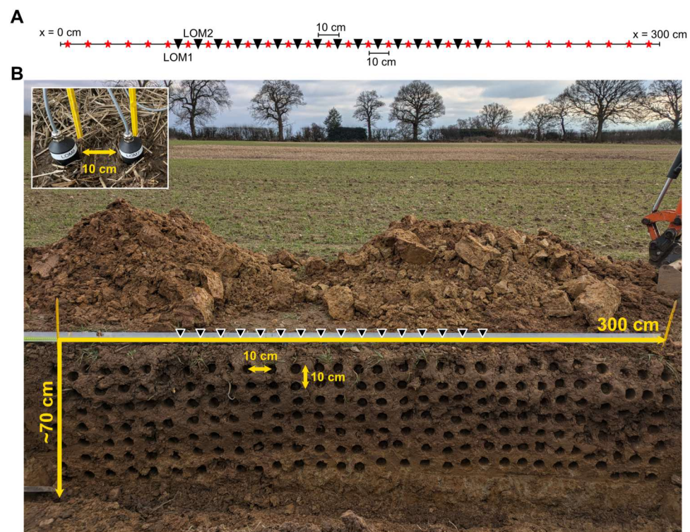
Figure 2. A Schematics of experimental set-up. In total 16 instruments were used (black inverted triangles). The red stars show the hammer strike location. B Photograph of the detailed soil sampling which was conducted right beneath the seismic experiments (black inverted triangles with white rim show approximate location of the geophones). Horizontal yellow line measures the extend of the trench (300 cm), vertical yellow line measures the depth of the trench. In total 210 soil samples were taken, with approximately 10 cm spacing between them, and analysed for each experimental treatment. Inlay shows zoom of LOM instruments during experiment.
