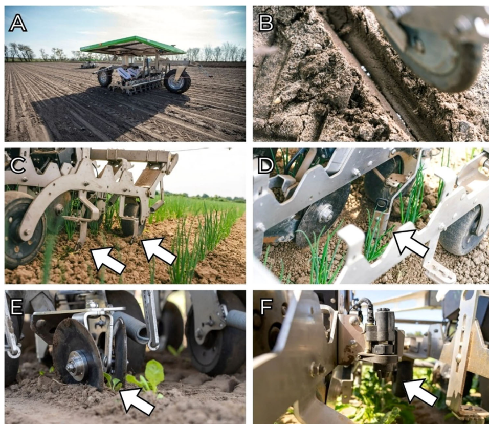
FIGURE 1 (A) The FarmDroid FD20 seeding and weeding robot; (B) crop seeding; (C) inter-row weeding hoes; (D) intra-row weeding knives; (E) close-to-crop weed cutting discs; (F) optional spot-spraying. Images are used courtesy of FarmDroid (2025).
