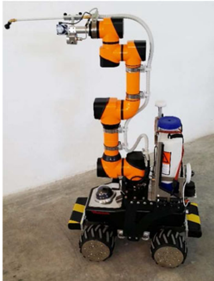
Figure 5. Precision light-weight pesticide spraying robotic arm mounted to a mobile base [71].
